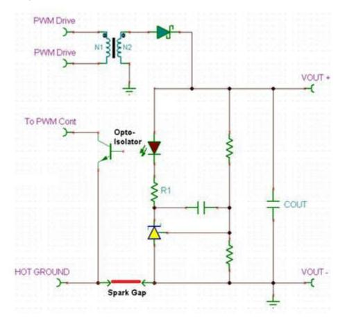
Figure 1-5. Spark Gap Protection Components; the Red Line Represents an Electric Arc
