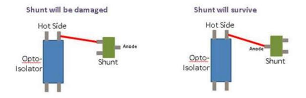
Figure 1-4. Layout Matters. the Red Line Represents an Electric Arc.
