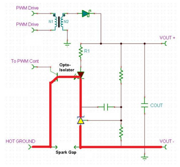
Figure 1-2. The Red Line Is the ESD Path, with an Electric Arc across Optical-isolator Leads
