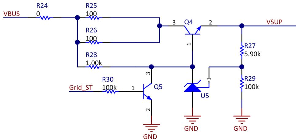
Figure 2. Charger for Super Capacitor
