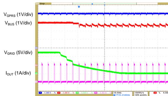
Figure 6. Transition Waveform When Grid Power is Off
