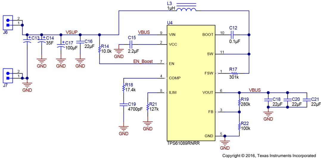
Figure 3. Schematic of Boost Converter Solution
