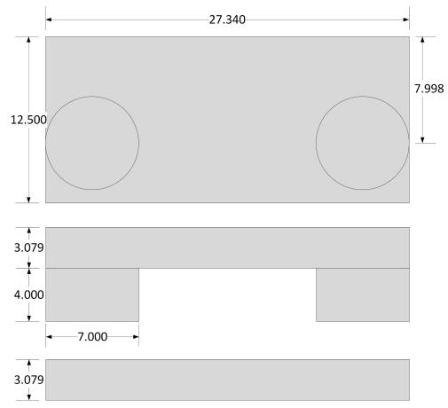
Figure 1-2. Transformer Core
