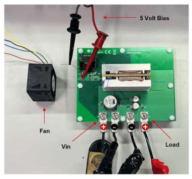
Figure 1-4. Test Connections
