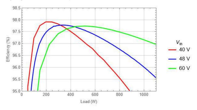
Figure 2-1. Efficiency Graph
