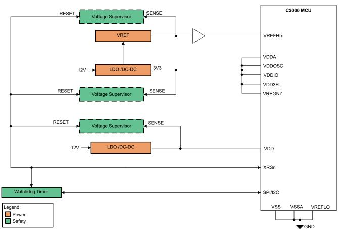
Figure 3-1. Non-Safety: MCU With External VREFHI and External VREG
