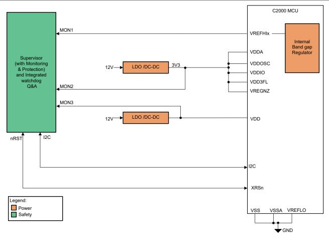
Figure 2-4. ASILB: MCU With Internal VREFHI and External VREG
