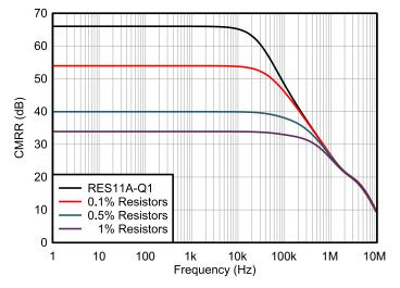
Figure 3-2. Minimum CMRR of Difference Amplifier with RES11A-Q1 vs Discrete Resistors OPA387, Gain = 1 V/V
