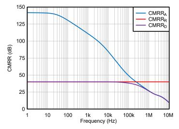
Figure 2-4. Resistor and Op-Amp Contributions to Effective CMRR of Difference Amplifier OPA387 with 0.5% Tolerance Resistors
