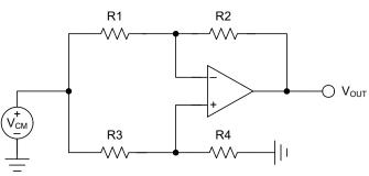
Figure 4-4. Superposition: Common-Mode
