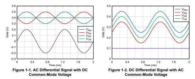
In practical electrical circuits the common-mode voltage is not perfectly removed from the differential signal, however it can be significantly attenuated. The magnitude of the common-mode attenuation is determined by various non-idealities in the circuit, as discussed in the following sections.
