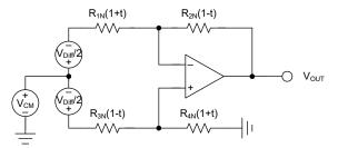
Figure 5-1. Worst-Case Resistor Matching of Difference Amplifier Circuit
