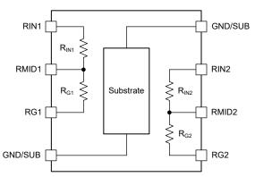
Figure 3-1. RES11A-Q1 Precision Matched Resistor Divider Pair
