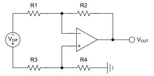
Figure 4-3. Superposition: Differential-Mode
