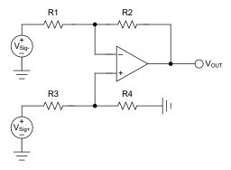
Figure 2-1. Difference Amplifier Circuit
