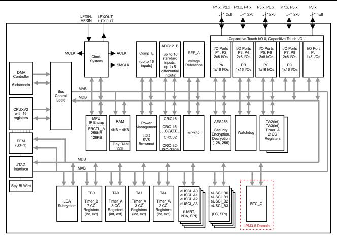
A. The device has 8KB of RAM, and 4KB of the RAM is shared with the LEA subsystem. The CPU has priority over the LEA subsystem.
