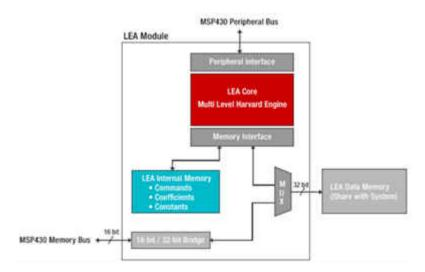
Figure 1. Simplified LEA block diagram
