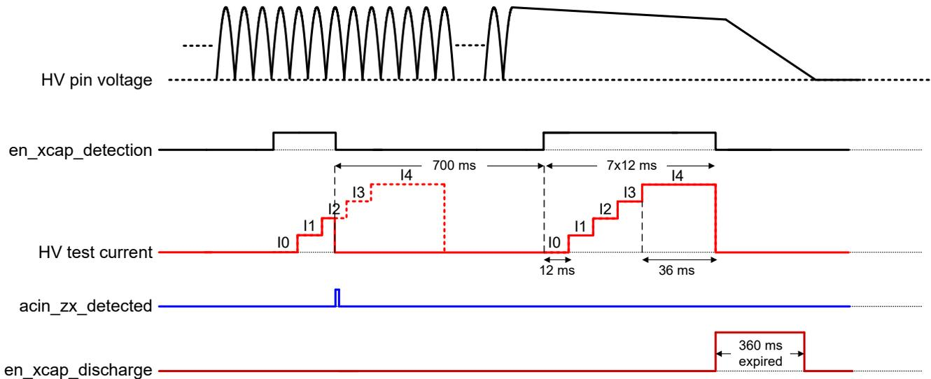
图 7-21. Zero Cross Detection Sequence HV Pin Only
