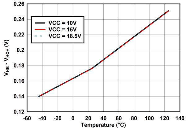
6-20. ( $V_{HB} - V_{HOH}$ ) vs Temperature
