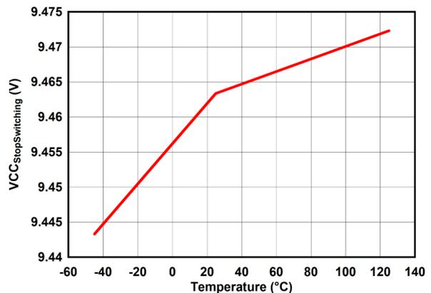
6-24.  $V_{CC\_StopSwitching}$  vs Temperature
