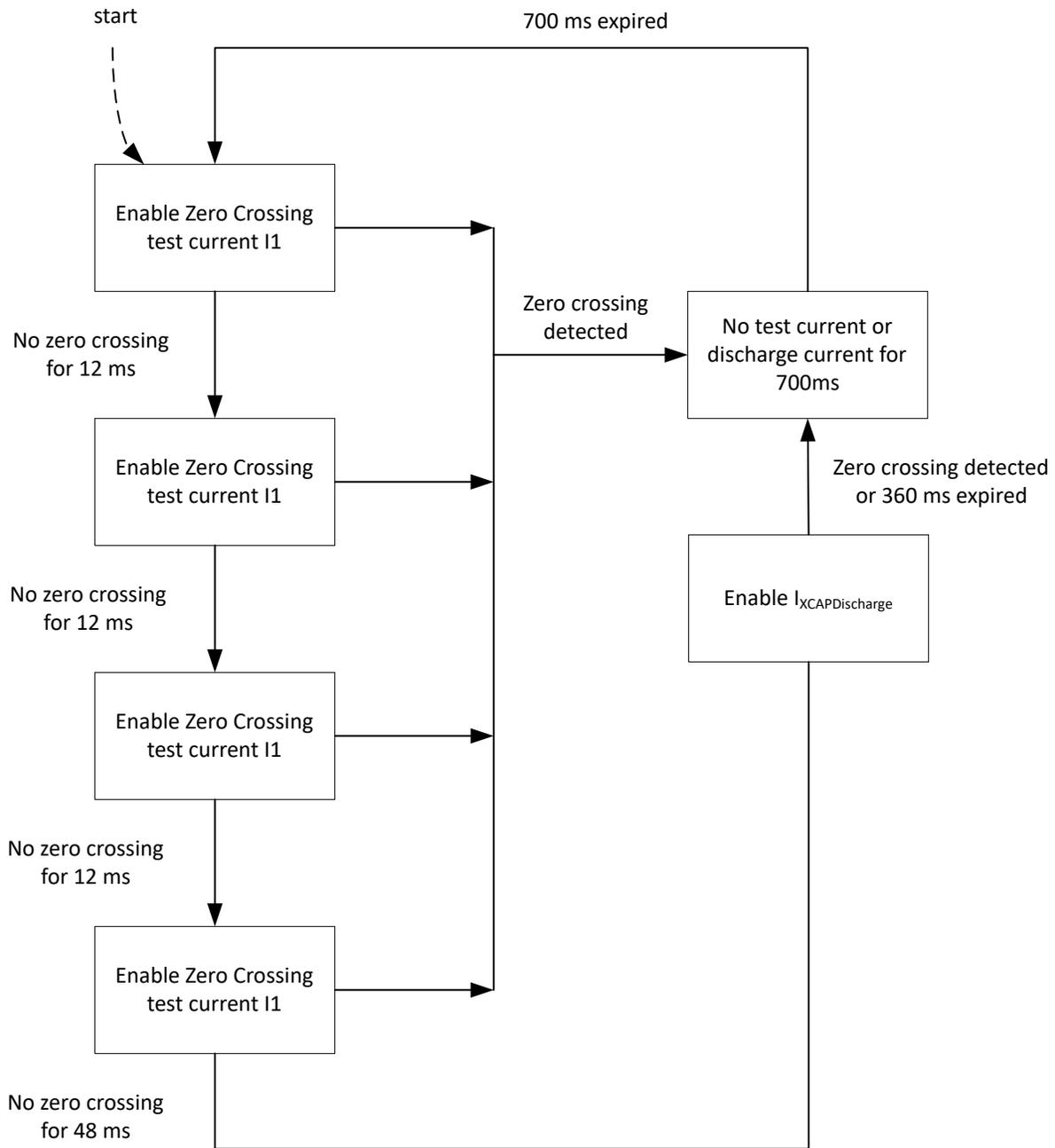
図 7-22. AC ZCD and X-Capacitor Discharge Flow Chart
