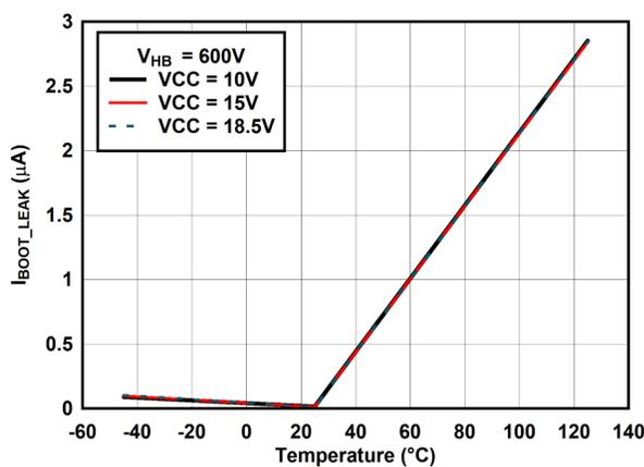
6-5. I<sub>BOOT\_LEAK</sub> vs Temperature
