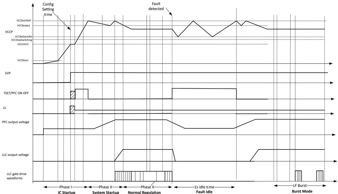
図 7-13. Startup Sequence for “HV Startup” Feature Enabled
