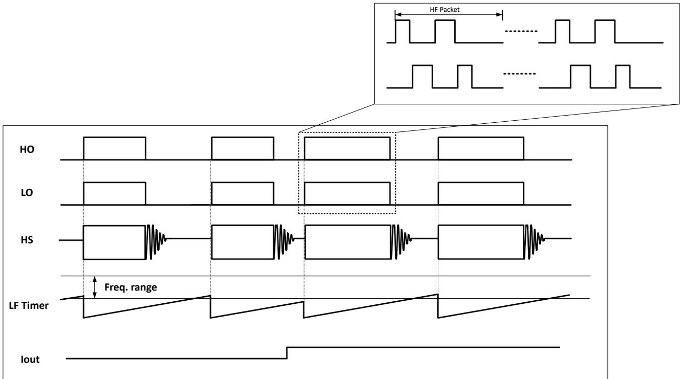
図 7-18. Packet Size Regulation Inside LF Burst
