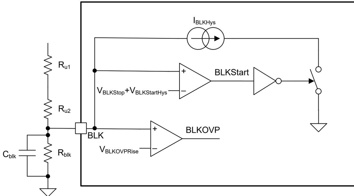
図 7-6. BLK Pin Input Voltage Sensing Architecture
