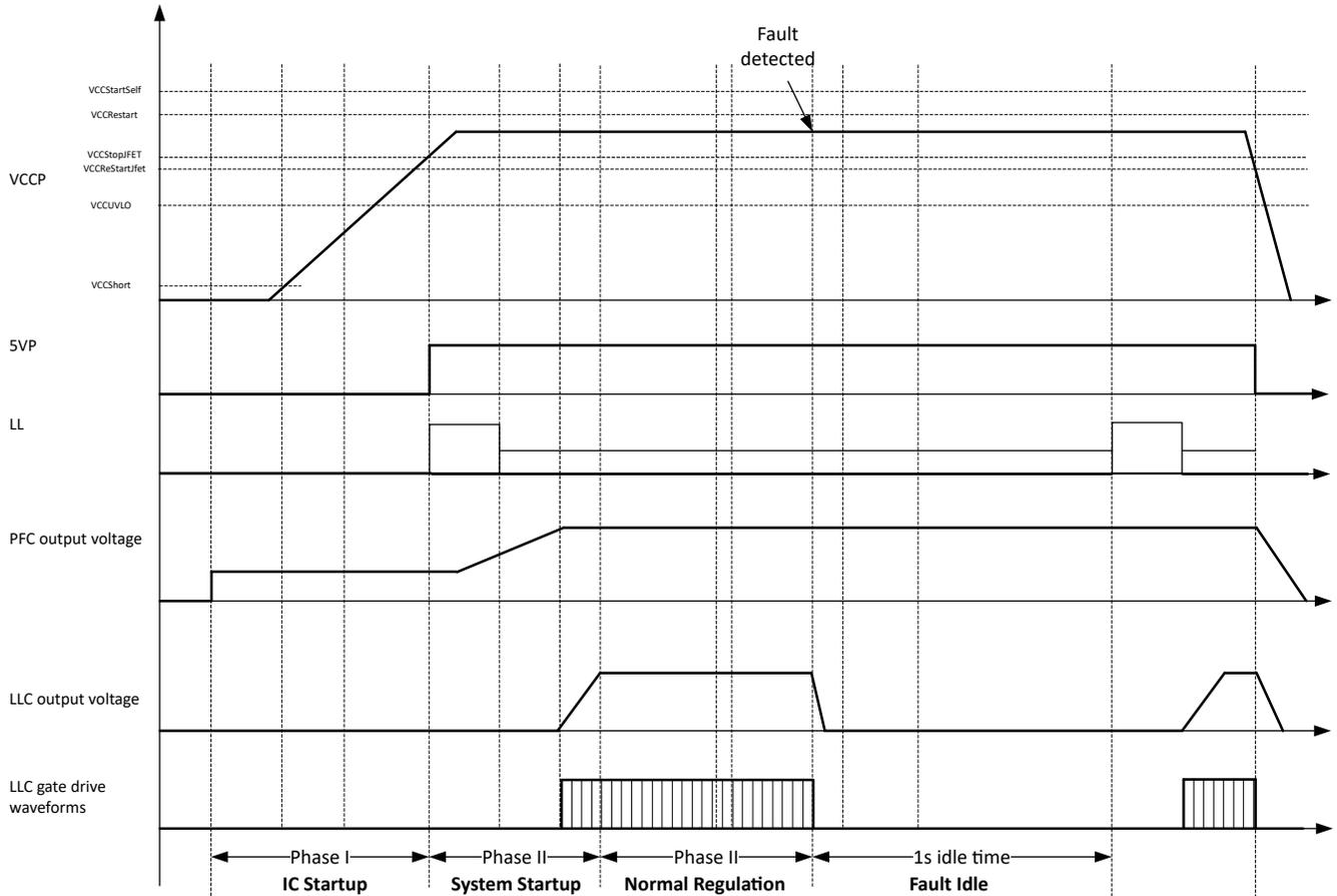
図 7-14. Startup Sequence for “HV Startup” Feature Disabled
