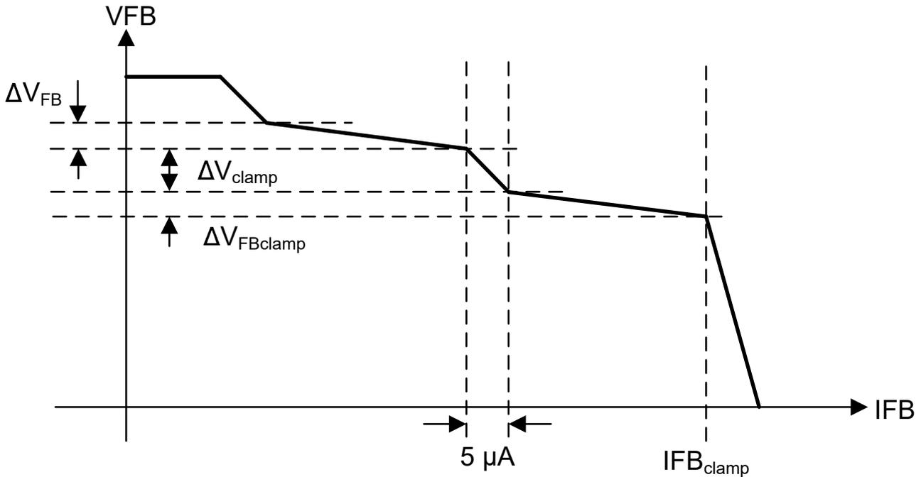
図 7-5. FB Pin Voltage vs FB Pin Current
