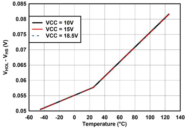
6-19. ( $V_{HOL} - V_{HS}$ ) vs Temperature
