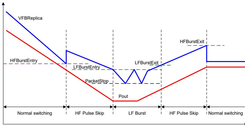
☒ 7-19. Burst Mode Determination from *FB Replica* Comparators
