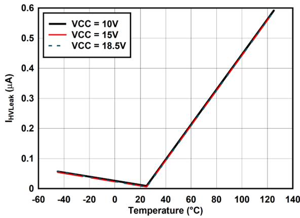
6-3. I<sub>HVLeak</sub> vs Temperature
