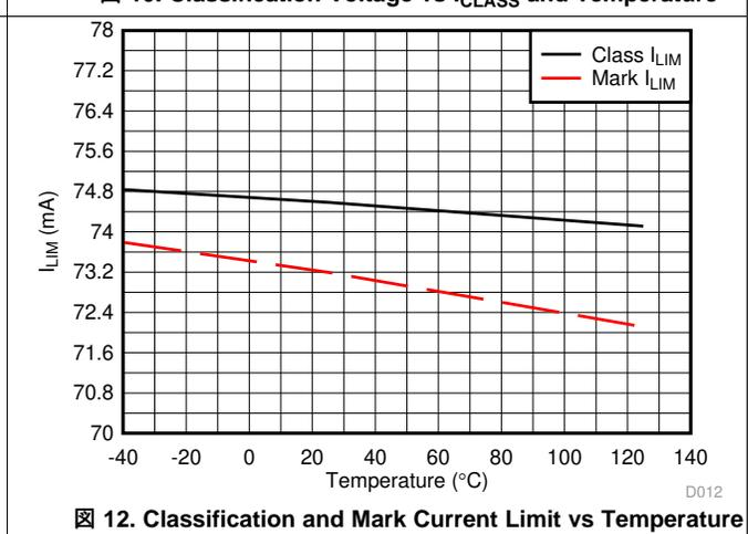
Figure 12. Classification and Mark Current Limit vs Temperature
