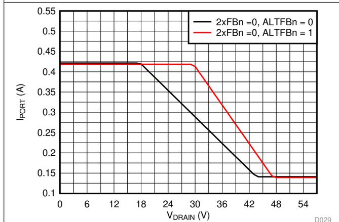
Figure 29. 1x Mode (2xFBn = 0) Current Foldback vs Drain Voltage
