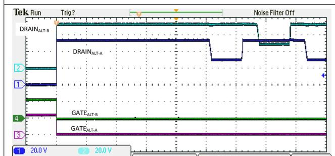
图 129. 4-Pair Backoff Due to 4PPCut Fault
