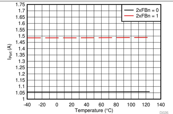
Figure 26. I<sub>SHORT</sub> Threshold vs Temperature
