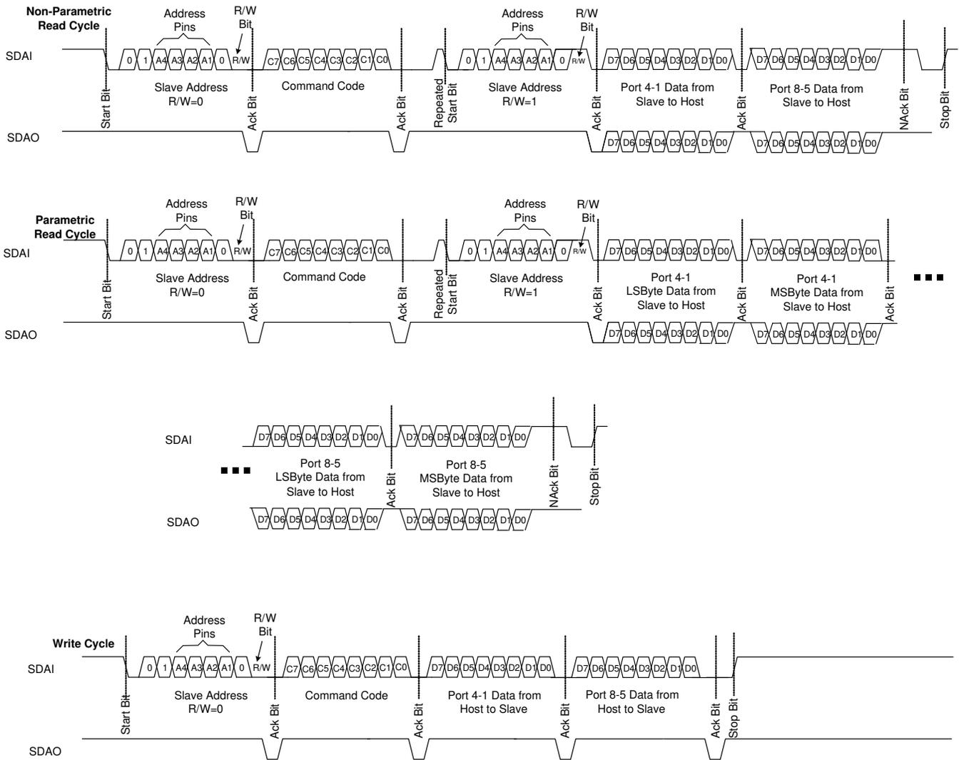
FIG 44. I<sup>2</sup>C interface Read and Write Protocol – Configuration B
