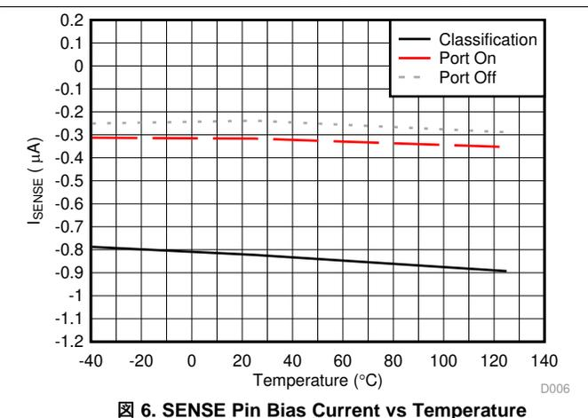
Figure 6. SENSE Pin Bias Current vs Temperature
