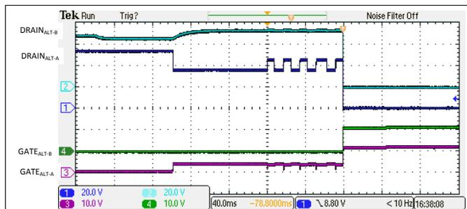
Figure 143. 4-Pair Single Signature Turn On with 5-Finger Classification and Turn On
