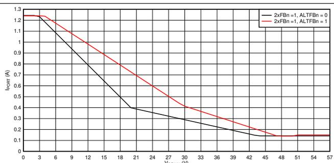
**☒ 117. 2x Mode (2xFBn = 1) Foldback Curves, I<sub>PORT</sub> vs V<sub>DRAIN</sub>**
