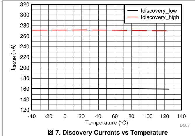
Figure 7. Discovery Currents vs Temperature
