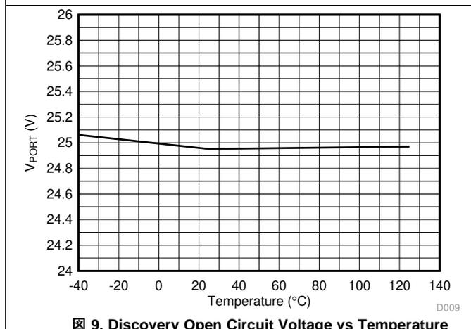
Figure 9. Discovery Open Circuit Voltage vs Temperature
