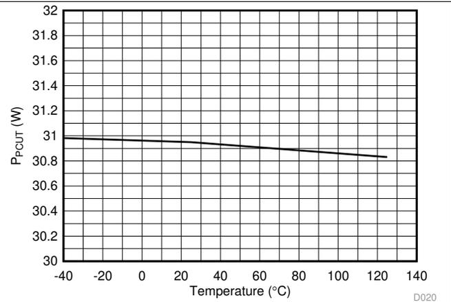
图 20. 2-Pair PCut Threshold (30W) vs Temperature
