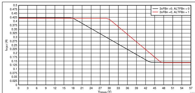
**☒ 116. 1x Mode (2xFBn = 0) Foldback Curves, I<sub>PORT</sub> vs V<sub>DRAIN</sub>**
