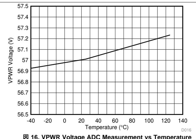
Figure 16. VPWR Voltage ADC Measurement vs Temperature
