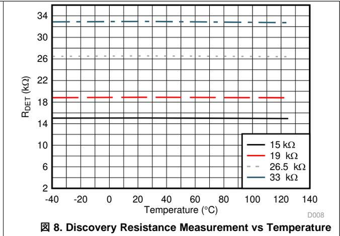
Figure 8. Discovery Resistance Measurement vs Temperature
