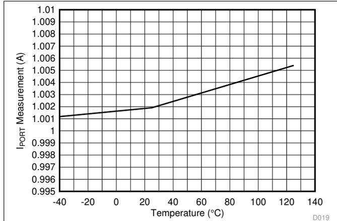
图 19. Port Current ADC Measurement (1 A) vs Temperature
