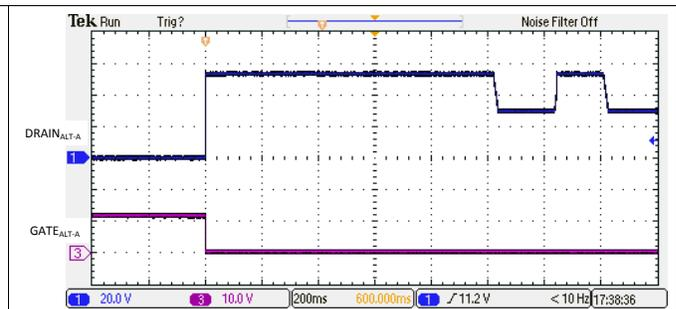
图 126. 2-Pair Backoff due to PCut Fault
