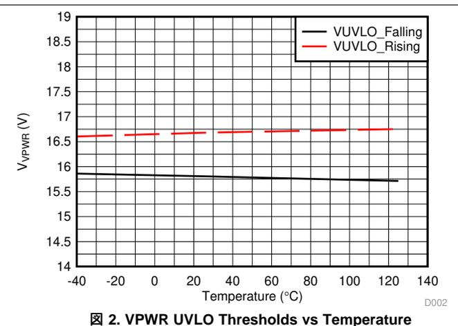
Figure 2. VPWR UVLO Thresholds vs Temperature
