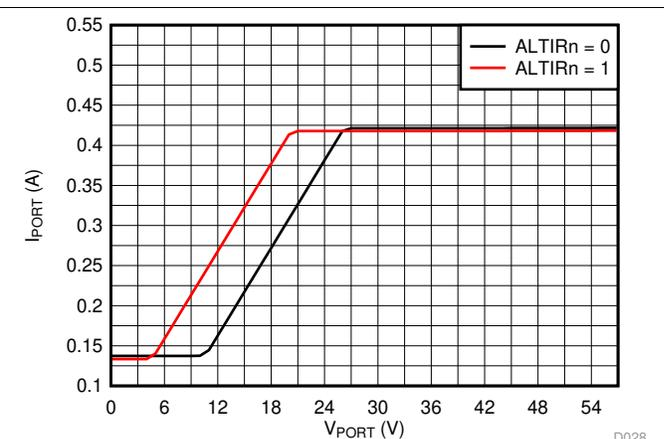
Figure 28. Inrush Current Foldback vs Port Voltage
