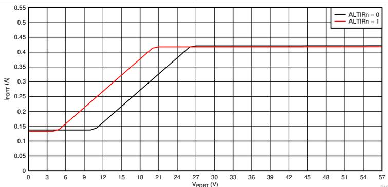
**☒ 118. Inrush Foldback Curves, I<sub>PORT</sub> vs V<sub>PORT</sub>**
