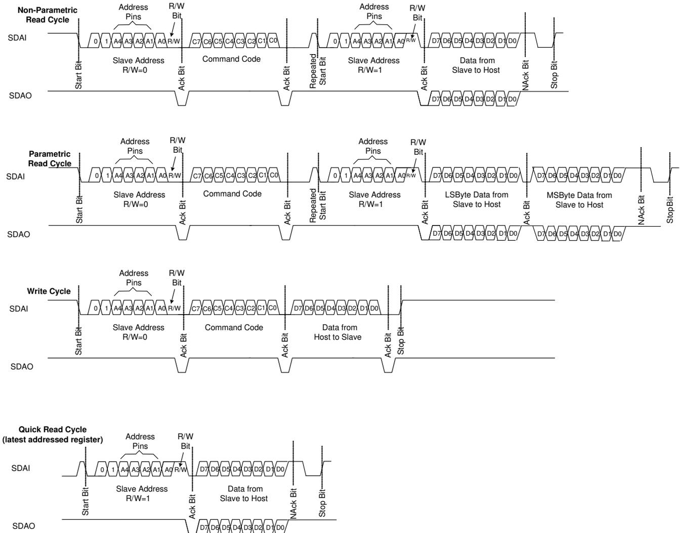
⊠ 43. I<sup>2</sup>C interface Read and Write Protocol – Configuration A
