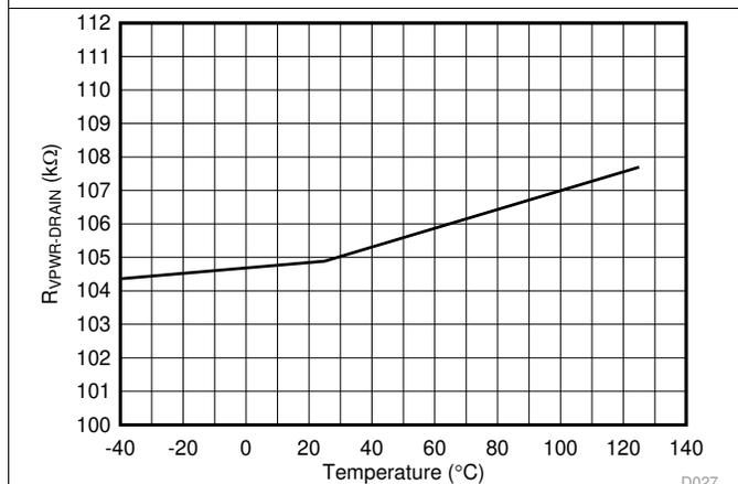
Figure 27. R<sub>OFF</sub> (VPWR to DRAIN) vs Temperature
