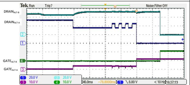
Figure 142. 4-Pair Single Signature Turn On with 4-Finger Classification and Turn On
