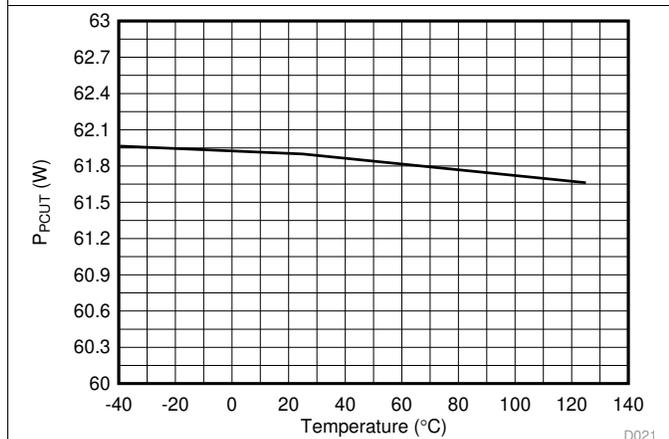
图 21. 4-Pair PCut Threshold (60W) vs Temperature
