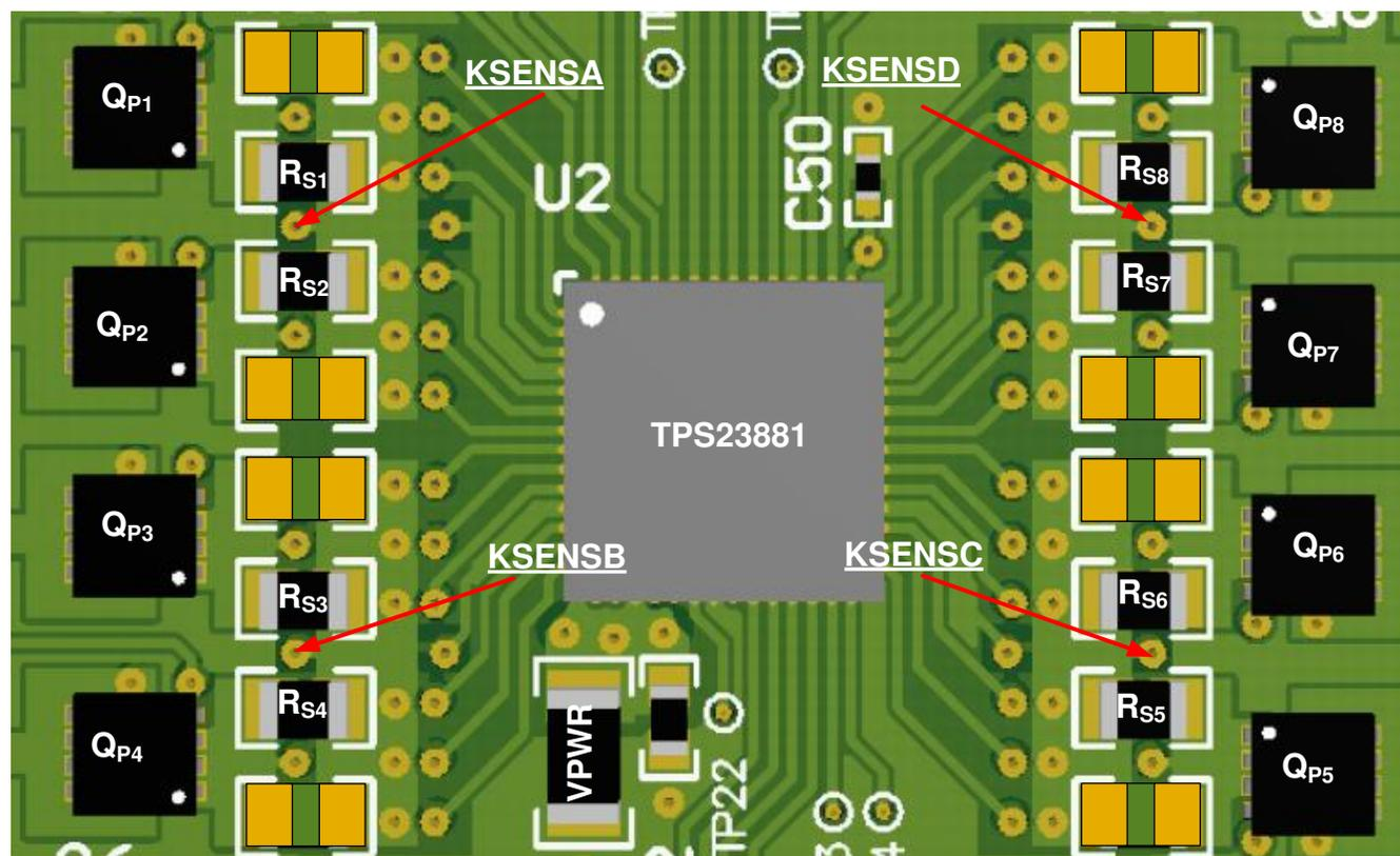
Note: PCB layout includes footprints for optional parallel  $R_{SENSE}$  resistors
