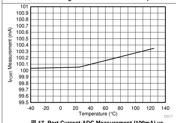
Figure 17. Port Current ADC Measurement (100mA) vs Temperature
