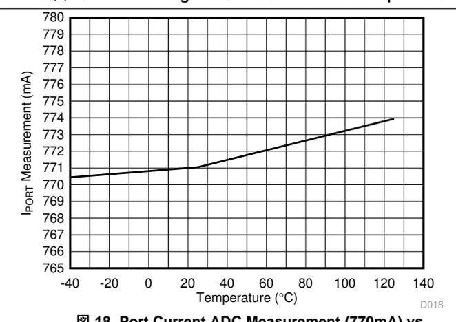
Figure 18. Port Current ADC Measurement (770mA) vs Temperature
