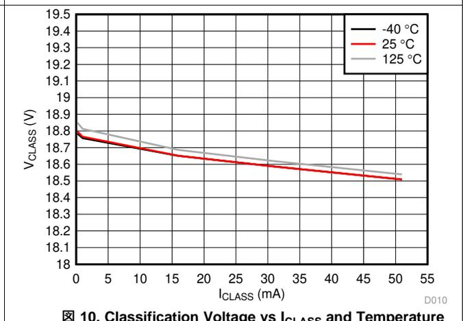
Figure 10. Classification Voltage vs  $I_{CLASS}$  and Temperature
