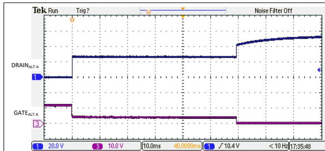
图 125. 2-Pair  $I_{LIM}$  Foldback and Turn Off
