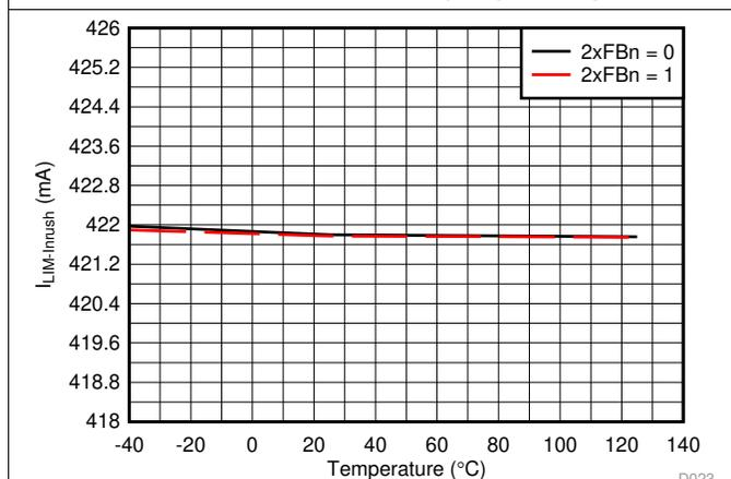
图 23. Inrush Current Limit vs Temperature
