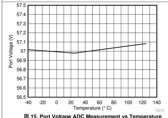
Figure 15. Port Voltage ADC Measurement vs Temperature
