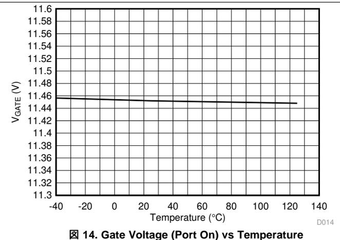
Figure 14. Gate Voltage (Port On) vs Temperature
