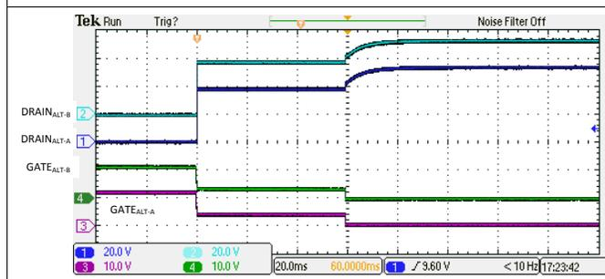
图 127. 4-Pair  $I_{LIM}$  Foldback and Turn Off
