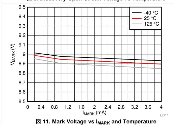
Figure 11. Mark Voltage vs  $I_{MARK}$  and Temperature
