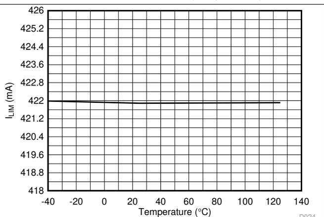
图 24. 1x Mode (2xFBn = 0) Current Limit vs Temperature
