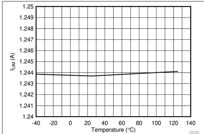
Figure 25. 2x Mode (2xFBn = 1) Current Limit vs Temperature
