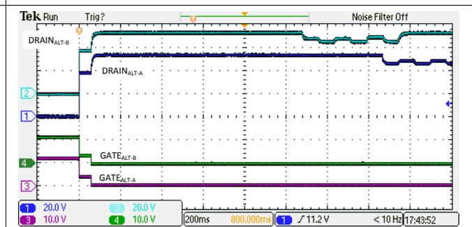
图 128. 4-Pair Backoff Due to  $I_{LIM}$  Fault
