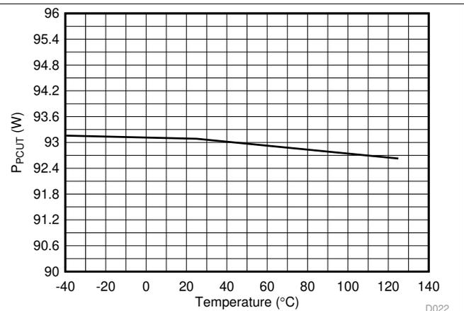
图 22. 4-Pair PCut Threshold (90W) vs Temperature
