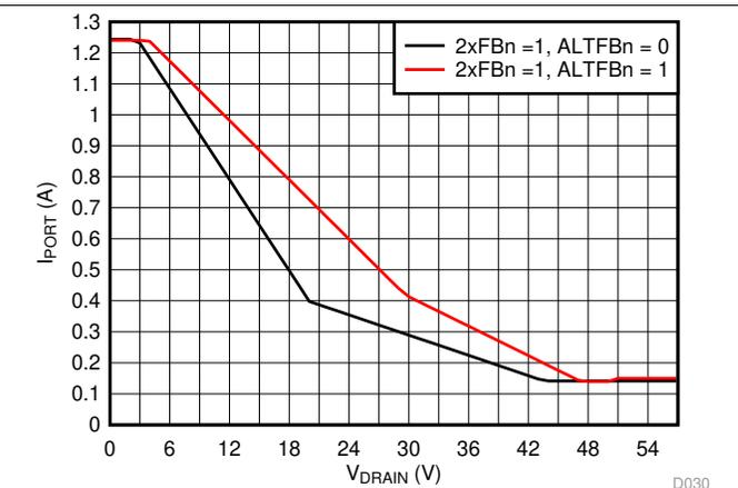
Figure 30. 2x Mode (2xFBn = 1) Current Foldback vs Drain Voltage
