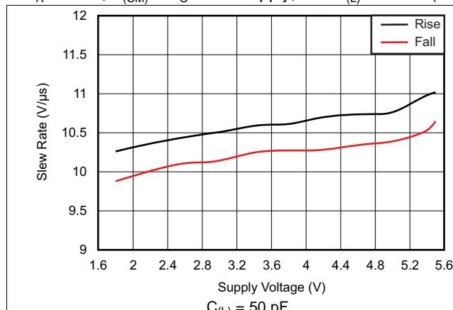
**Figure 25. Slew Rate vs Supply Voltage**
