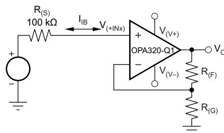
**Figure 40. Noise as a Result of  $I_{(BIAS)}$**
