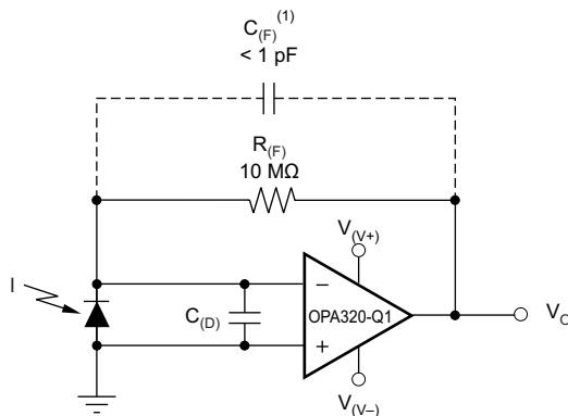
(1)  $C_{(FB)}$  is optional to prevent gain peaking.  $C_{(FB)}$  includes the stray capacitance of  $R_{(FB)}$ .
