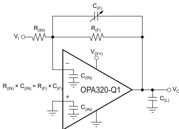
NOTE: Where  $C_{(IN)}$  is equal to the OPAX320-Q1 input capacitance (approximately 9 pF) plus any parasitic layout capacitance.
