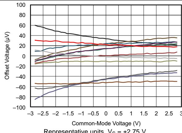
Figure 3. Offset Voltage vs Common-Mode Voltage
