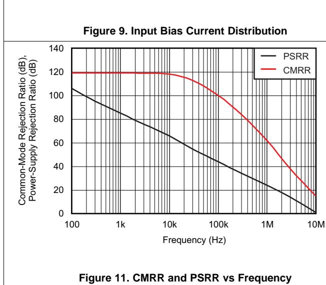
**Figure 11. CMRR and PSRR vs Frequency**
