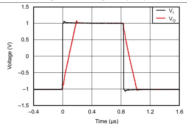
**Figure 28. Large-Signal Step Response vs Time**
