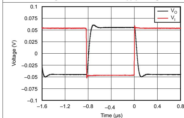
**Figure 27. Small-Signal Step Response**
