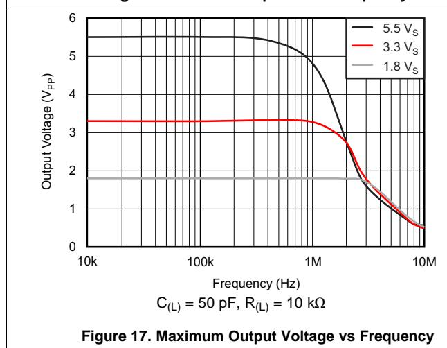
**Figure 17. Maximum Output Voltage vs Frequency**
