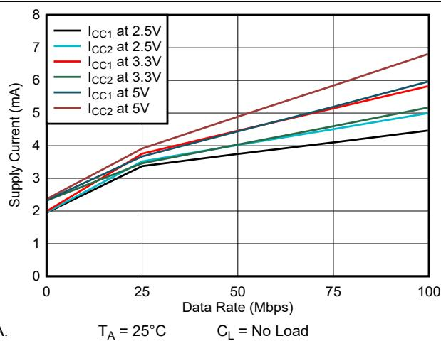
図 6-8. ISO7731 Supply Current vs Data Rate (With No Load)
