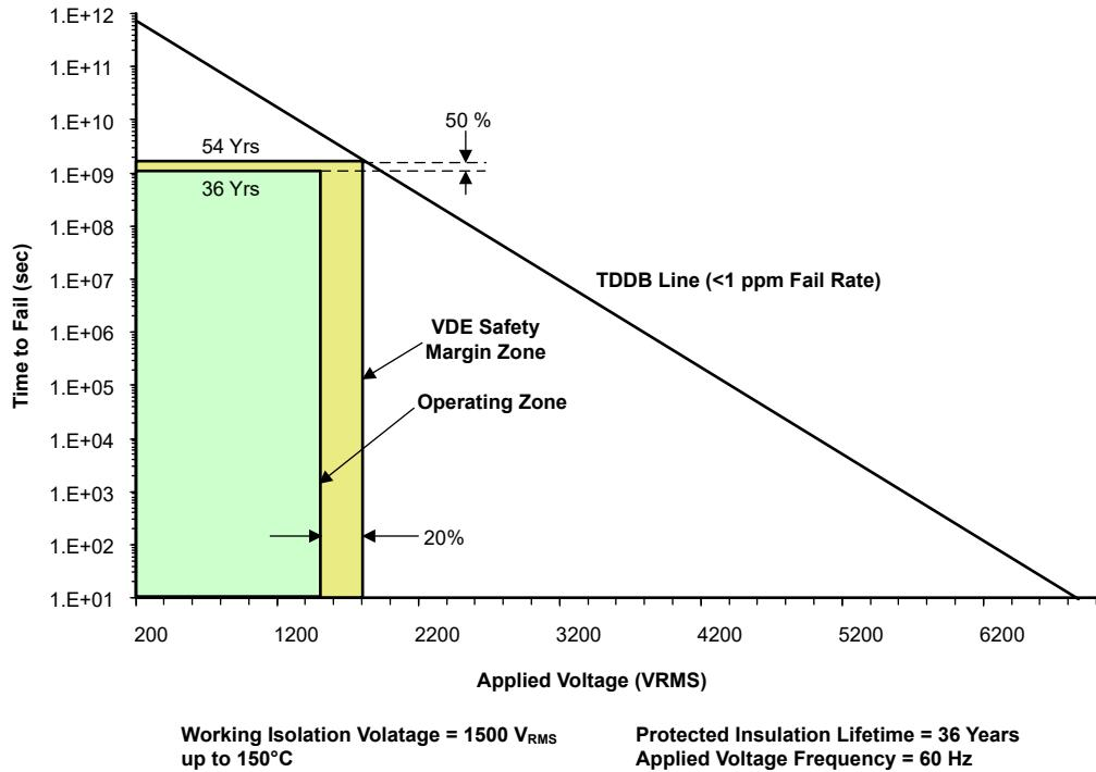
図 9-8. Insulation Lifetime Projection Data
