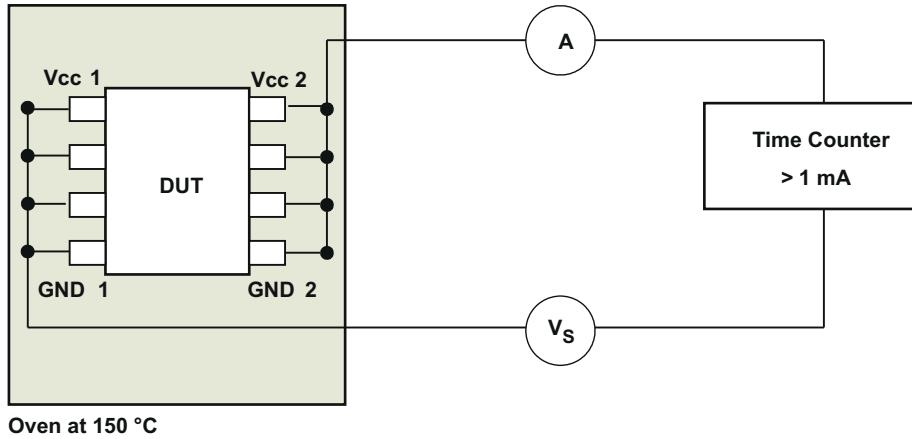
図 9-7. Test Setup for Insulation Lifetime Measurement
