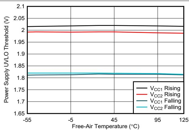
**図 6-11. Power Supply Undervoltage Threshold vs Free-Air Temperature**
