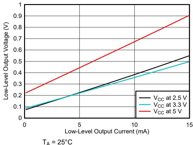
**図 6-10. Low-Level Output Voltage vs Low-Level Output Current**
