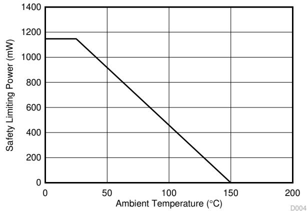
図 6-4. Thermal Derating Curve for Safety Limiting Power per VDE for DBQ-16 Package
