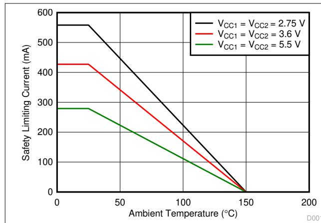
**图 6-1. Thermal Derating Curve for Safety Limiting Current per VDE for DW-16 Package**
