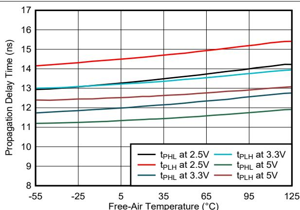
**図 6-12. Propagation Delay Time vs Free-Air Temperature**
