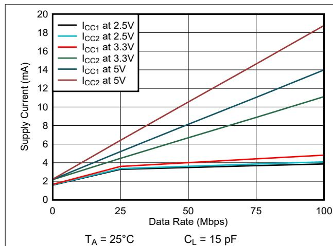
図 6-5. ISO7730 Supply Current vs Data Rate (With 15-pF Load)
