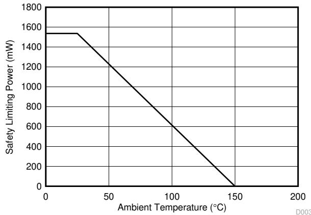
図 6-3. Thermal Derating Curve for Safety Limiting Power per VDE for DW-16 Package
