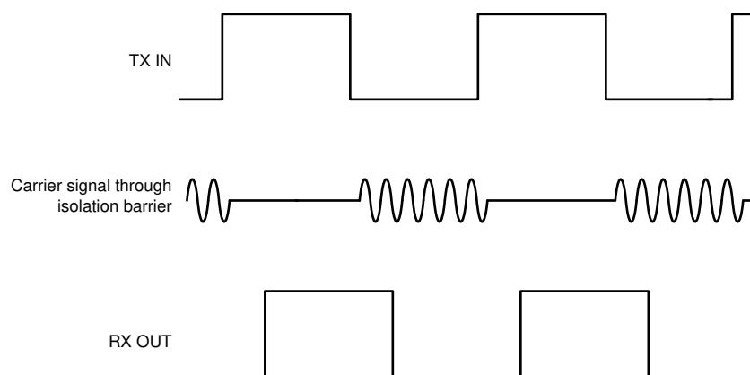
**図 8-2. On-Off Keying (OOK) Based Modulation Scheme**
