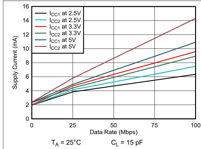
図 6-7. ISO7731 Supply Current vs Data Rate (With 15-pF Load)
