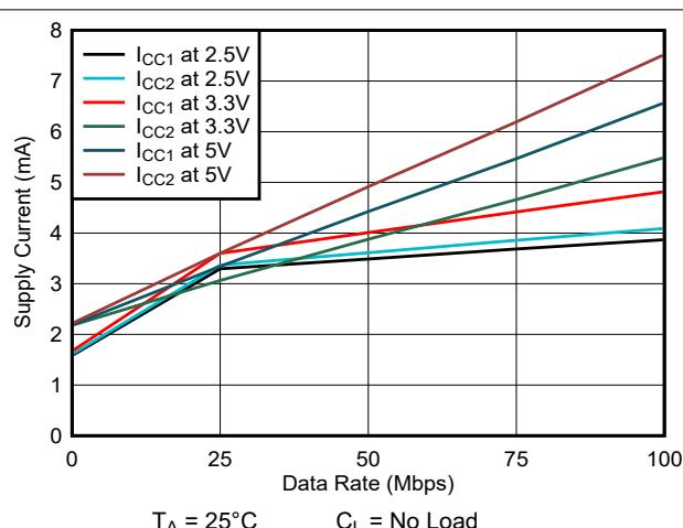
図 6-6. ISO7730 Supply Current vs Data Rate (With No Load)
