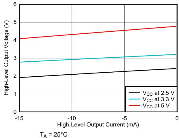
**図 6-9. High-Level Output Voltage vs High-level Output Current**
