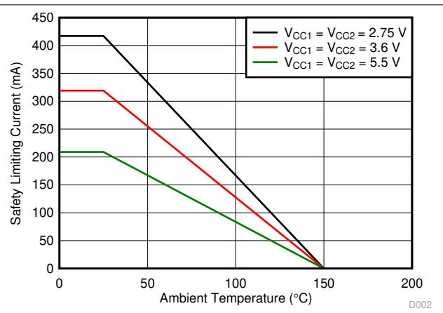
**图 6-2. Thermal Derating Curve for Safety Limiting Current per VDE for DBQ-16 Package**
